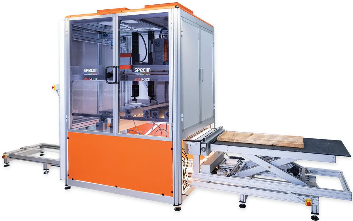
**SisuROCK is the most versatile imaging multicamera workstation for rapid and accurate core logging.**
