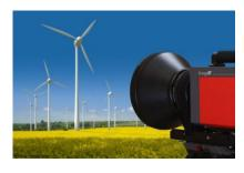
Highly thermally sensitive high-speed infrared cameras with high performance telephoto lenses are used to visualize the boundary layer condition of rotor blades in operation, in which the rotor blades and the measurement position are several hundred meters apart. These measurements deliver qualitative information regarding the transition location along the rotor blades, and allow comparisons between different operational states and conditions.
