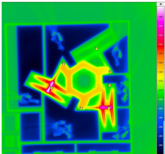
Fig. 1: Thermal image of a MEMS-controlled actuator with three degrees of freedom and thermal drives
