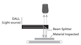
source light passes through the beam splitter/mirror, half of the light is directed to the object and the other half is directed to the camera. Even with today's high-intensity LEDs, the DALL is not effective for very fast production lines or applications where a high amount of intensity is required.
