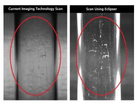
clear glass and plastic. Much as the rays of the sun form a halo effect during a total eclipse of the moon, the tiniest particle suspended in the material being scanned "glows" as the light passes behind it. The black background of the LED strip enhances contrast amplifying even sub-micron defects.
