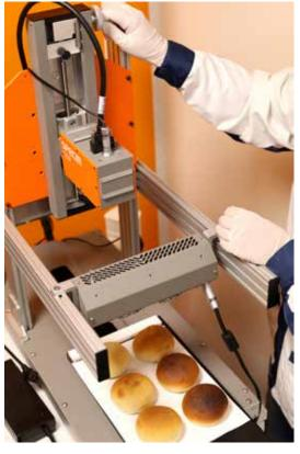
Since the camera works with the push-broom method, and images the target line by line, the target needs to move during the measurements. In our test setup, we mounted the FX10c camera on Specim Labscanner 40x20 to create the movement. However, a scanner is not a requirement, and the movement can be achieved for example by mounting the camera over a production line.
